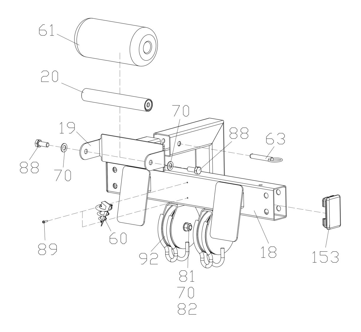
HG-5 Diagram 7: Cable Run Assembly Detail
