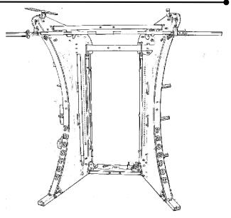
13. Rear Cover installation: Now before installing Right Locking Post Cover, feed Neon Wire Harness thru the access hole near bottom inside face of cover and plug into both the Neon Light Cross Brace Harness and Neon Light Wire Harness Reference diagram 7. Make sure Cover goes over the tabs for Machine Screws but goes between plates on top and bottom of the Cover. Tighten securely but be careful not to strip the screw heads.
